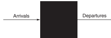
Figure D.15 Treating the I/O system as a black box. This leads to a simple but important observation: If the system is in steady state, then the number of tasks entering the system must equal the number of tasks leaving the system. This flow-balanced state is necessary but not sufficient for steady state. If the system has been observed or measured for a sufficiently long time and mean waiting times stabilize, then we say that the system has reached steady state.
