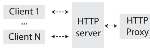
Figure 1: when using a proxy, the HTTP server serves requests by streaming them to a remote HTTP server (proxy). responses from the proxy are sent back to clients.
