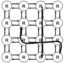
Assume that each router or link has a very small amount of buffer space and that each message can be arbitrarily long. Show a simple situation (with a drawing) in which messages are deadlocked and can make no further progress. *[Explain with no more than two sentences]:*
