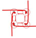
Answer: The simplest deadlock example is a set of four messages in a loop (as shown in the figure at the left). Each message is blocked attempting to make a counter-clockwise turn by a message utilizing the target channel.
