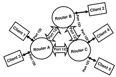
This problem will investigate the construction of a peer-to-peer communication network built. We will utilize instant messaging as our application on top of this network. As you see by the above figure, clients connect with individual routers. Messages transit from a source client to a destination client via one or more hops through a router.
