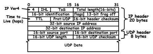
We will use UDP/IP for our implementation. The packet format is shown above. UDP/IP communication is *connectionless*. To communicate on a given port, an application simply *binds* a socket to that port, after which it can immediately begin sending and receiving messages on that
